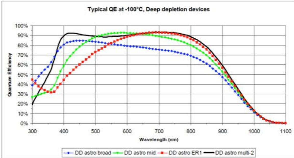
Figure 1: Quantum efficiency of the E2V CCD231-C6 deep depletion CCD
