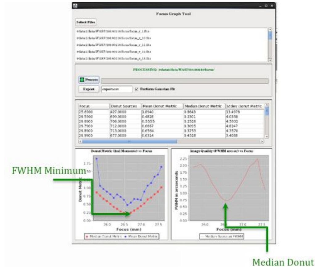
**Figure 12: Analysis of a classical “focus run” but using the donut metric based on the 2nd moments of out of focus donuts**
