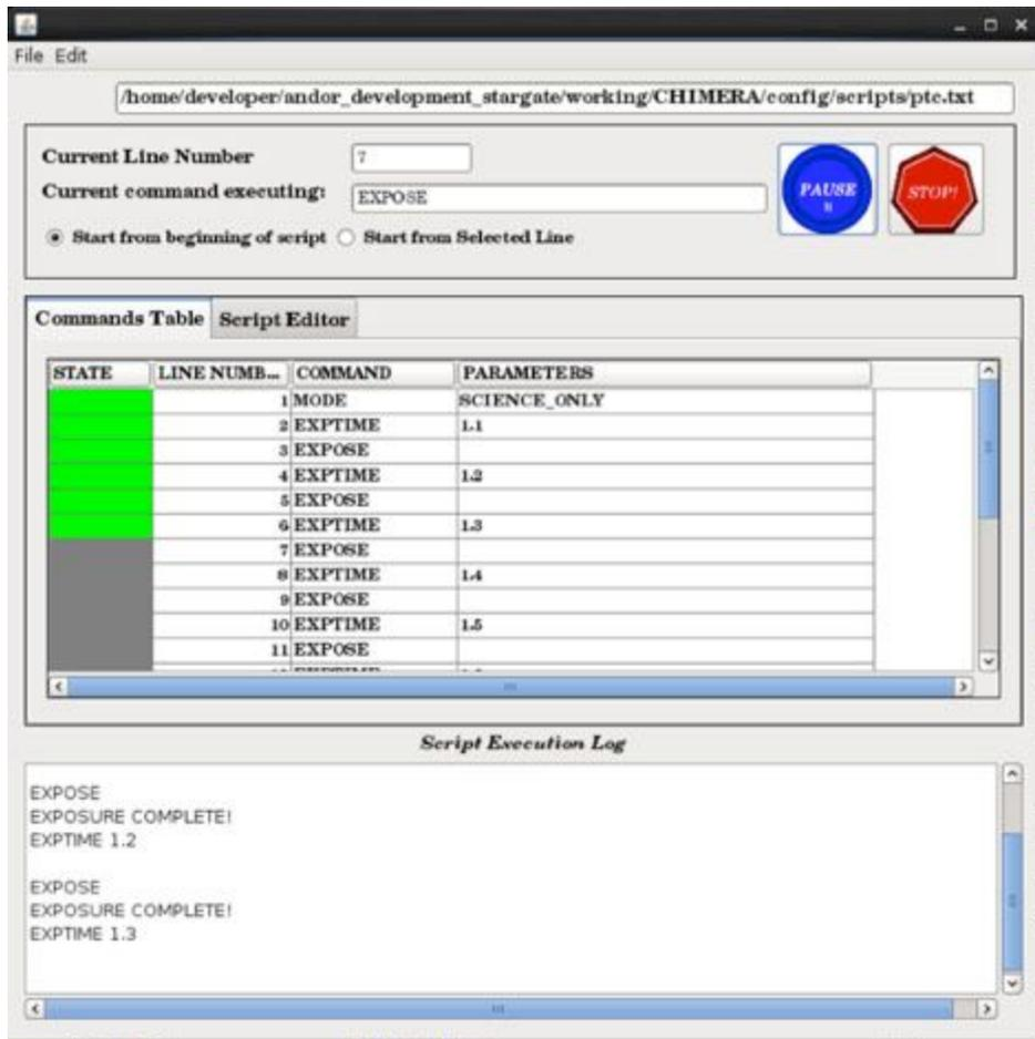
**Figure 9: WASP script execution control. Automating the taking of FLAT calibration images**
