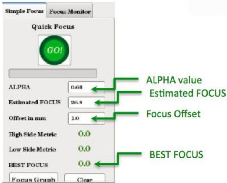
Figure 13: Using the “Quick Focus” tool
