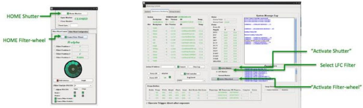
Figure 6: WASP mechanism controls, homing and activating the mechanisms
