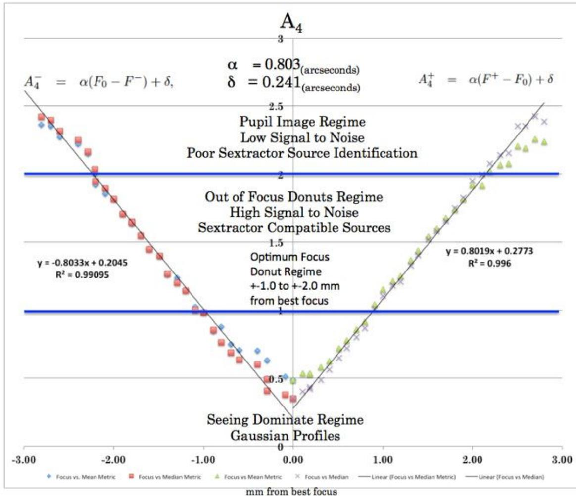
Figure 11: The “Donut” method of determining focus. Based on (A. Tokovinin and S. Heathcote 2006)
