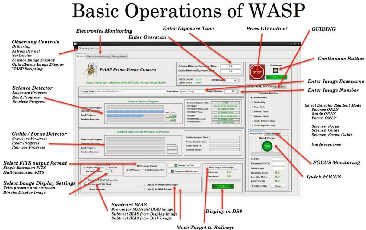
Figure 7: Basic operation of the WASP instrument
