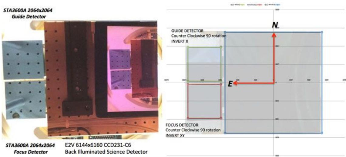
Figure 3: On-sky orientation of the science, guide and focus CCDs
