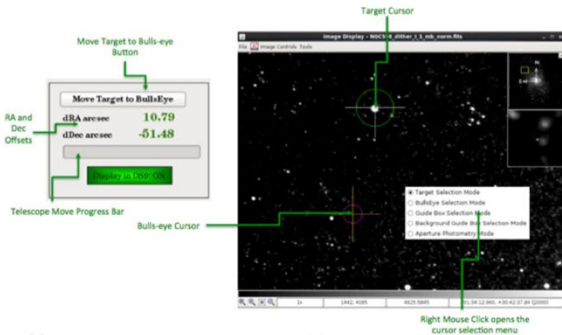
Figure 10: Using the "Target to Bullseye" control to position your target
