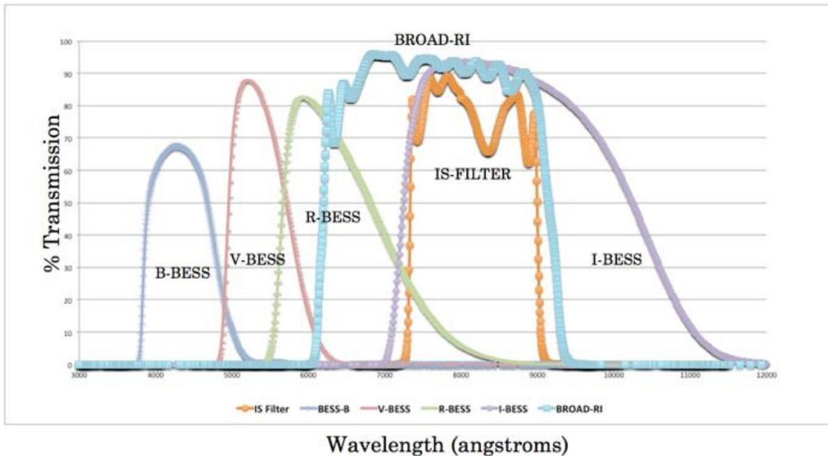
Figure 5: Transmission curves for Bessel filters and specialize variants
