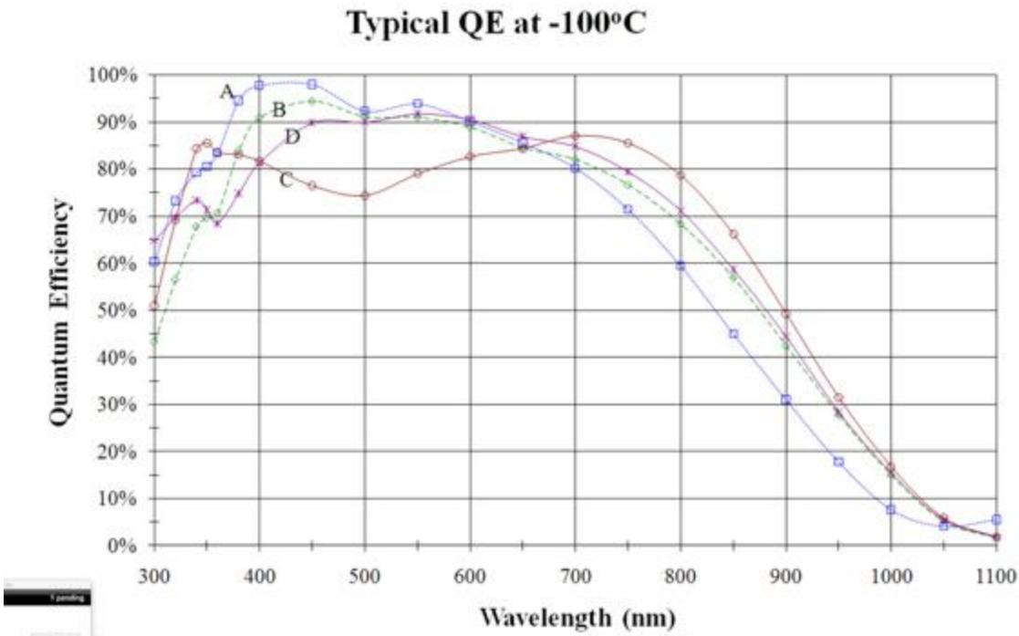
Figure 2: Quantum efficiency of the STA 3600A guide and focus CCDs
