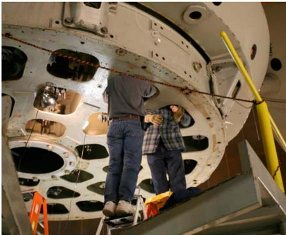
In case you don't know, the mirror supports "float" the 14.5-ton mirror to keep the force of gravity from deforming the glass no matter which way the telescope is pointed. Recently it became obvious that the supports were binding up and not consistently doing their job. Each of the 36 supports has over 1,000 parts. They were taken apart, cleaned and had their bearings replaced. Over 1,400 bearings were replaced on the project.
