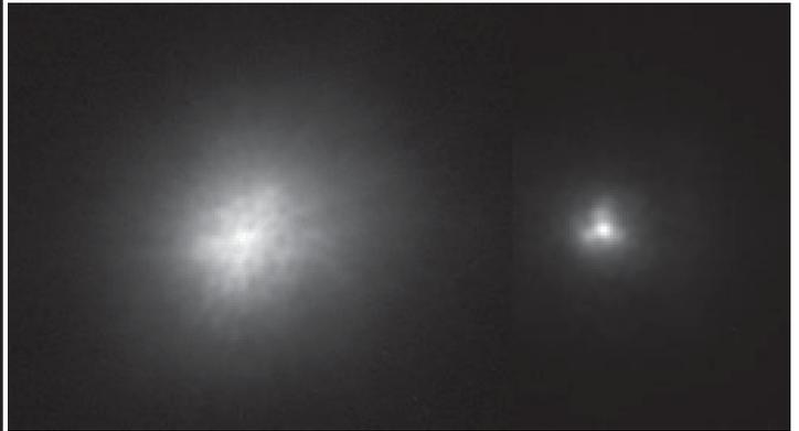
Last June marked an important milestone for the Palomar adaptive optics laser-guide star program. Above, left is an image that shows a blurred star taken through the 200-inch Hale Telescope. The image on the right reveals a much sharper image of the same star. It was the first such corrected image obtained at Palomar to make use of an artificial laser guide-star.
